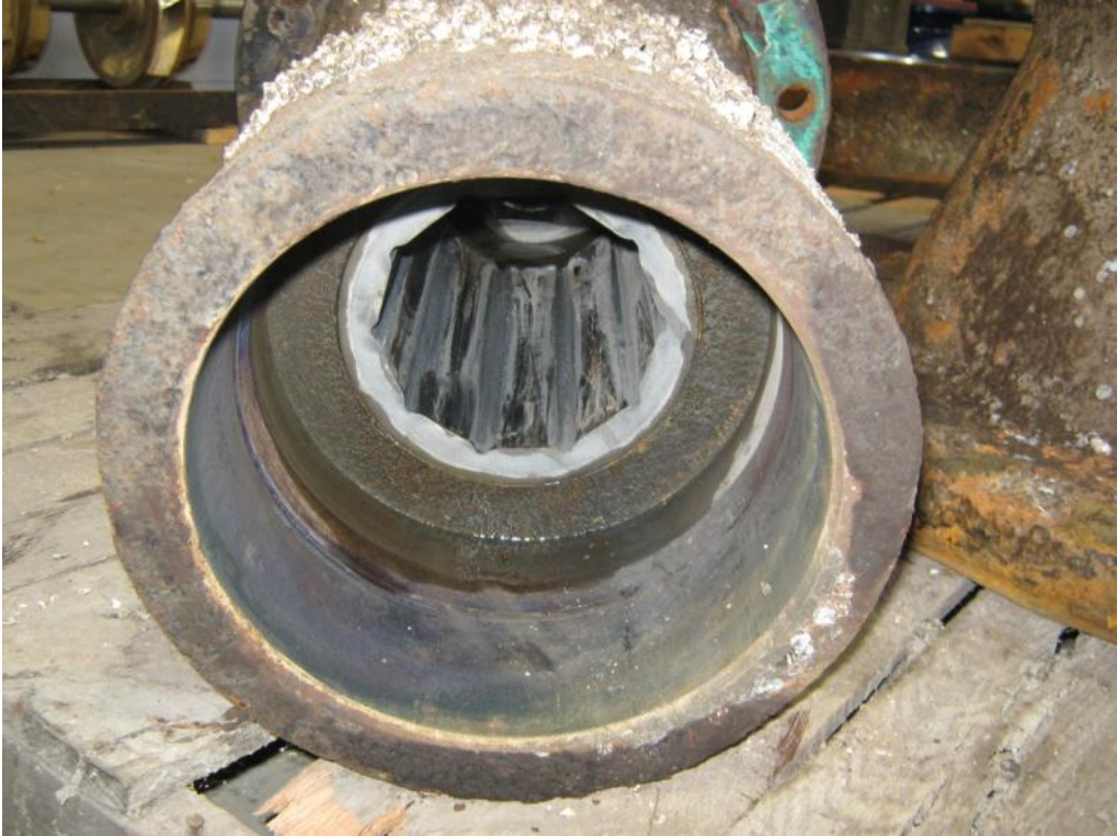
c. Stuff Box Bearing (Item 70) Worn/Replace. Bearing OD/Housing ID =6.122”
